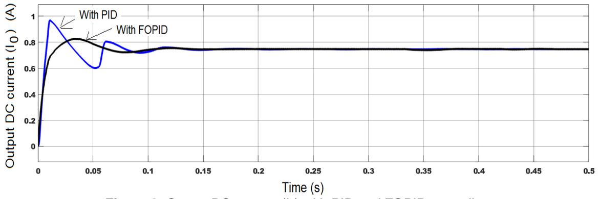
Figure 9. Output DC current ( $I_o$ ) with PID and FOPID controllers
