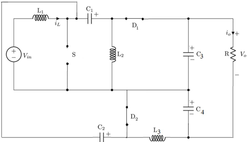
(c) **Figure 2.** Equivalent circuits of the suggested DC-DC converter - (a). Mode-I (b). Mode-II (c). Mode-III
