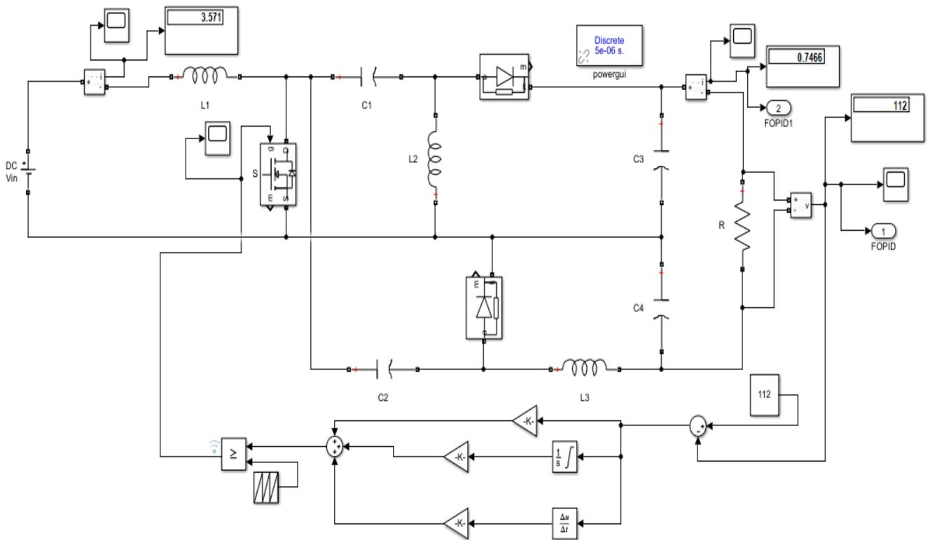
**Figure 4.** MATLAB / SIMULINK model of the proposed integrated DC-DC converter with FOPID controller
