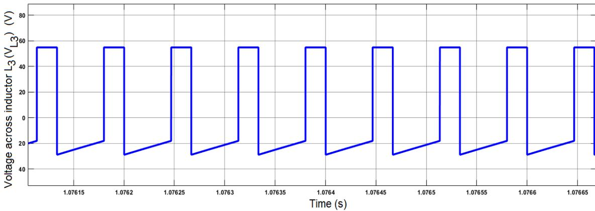
Figure 12. Voltage across inductor  $L_3$  ( $V_{L3}$ )
