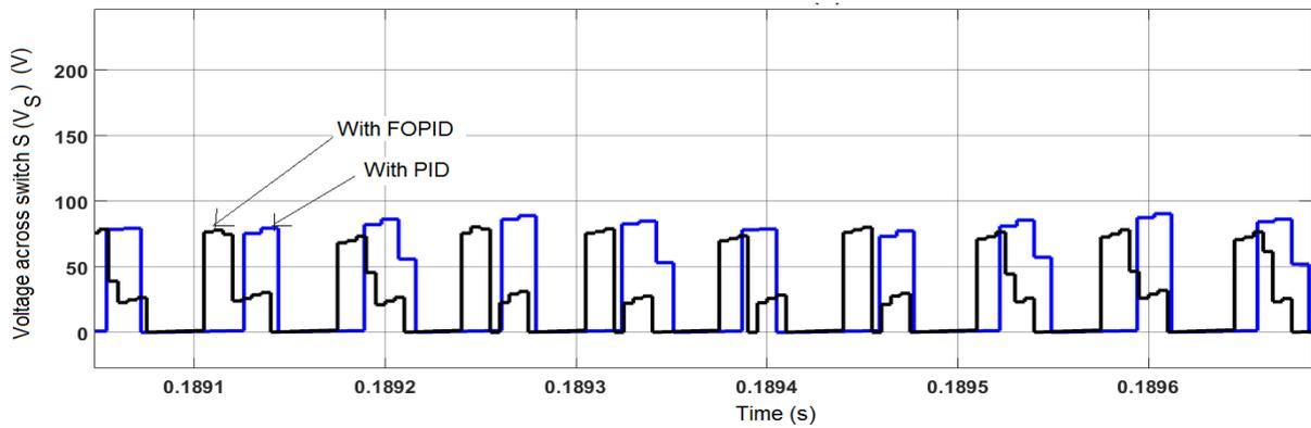
Figure 19. Voltage stress across switch S ( $V_s$ )
