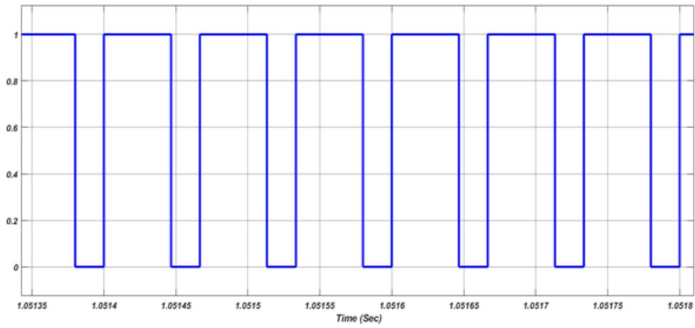
Figure 5. Gate pulse waveform for the switch S
