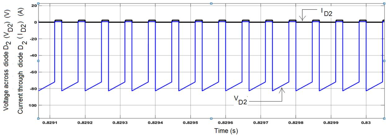
Figure 18. Voltage across diode D<sub>2</sub> ( $V_{D2}$ ) and Current through diode D<sub>2</sub> ( $I_{D2}$ )
