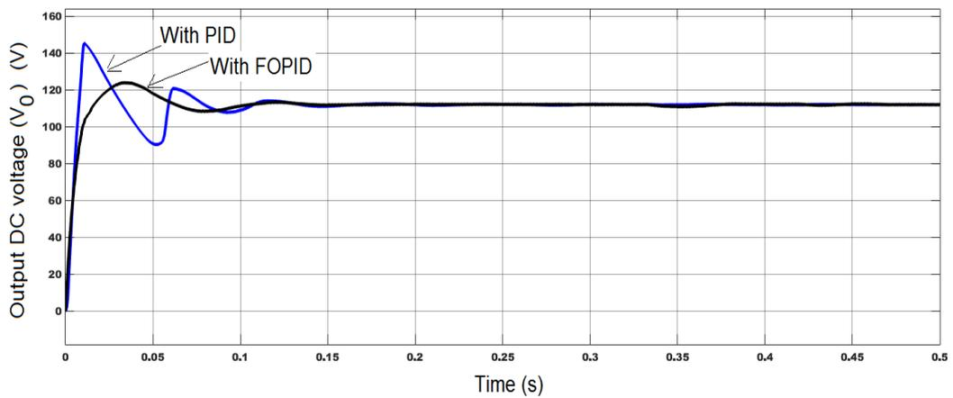
Figure 8. Output DC voltage ( $V_o$ ) with PID and FOPID controllers
