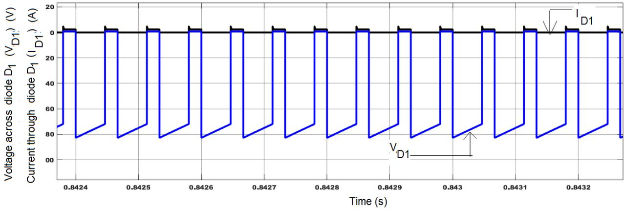
Figure 17. Voltage across diode D<sub>1</sub> ( $V_{D1}$ ) and Current through diode D<sub>1</sub> ( $I_{D1}$ )
