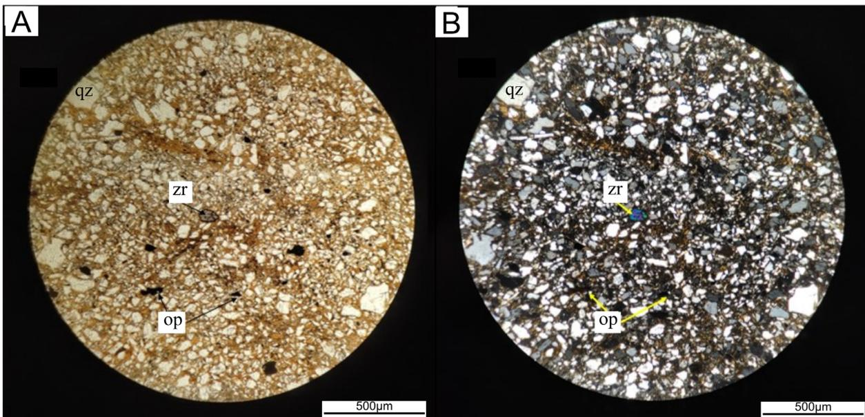
**Figure 4.** Microphotography of thin section, 10× magnification, of the immature sandy quartzose sediments from MAD-FSE003 (71 m), rich in angular quartz grain (qz), some opaque minerals (op) and rare zircon (zr) (A) under plane-polarized light and (B) under crossed-polarized light.
