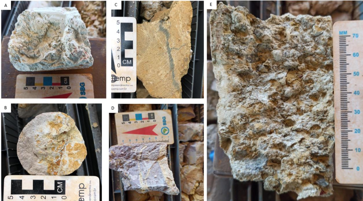
**Figure 3.** (A) White clay, massive; (B) clay with white and ochre massive portions and quartz pebble in small proportion; (C) material with manganiferous vein; (D) pink clay; (E) rounded pebble and cobble conglomerate, of mica schist and lateritic material.
