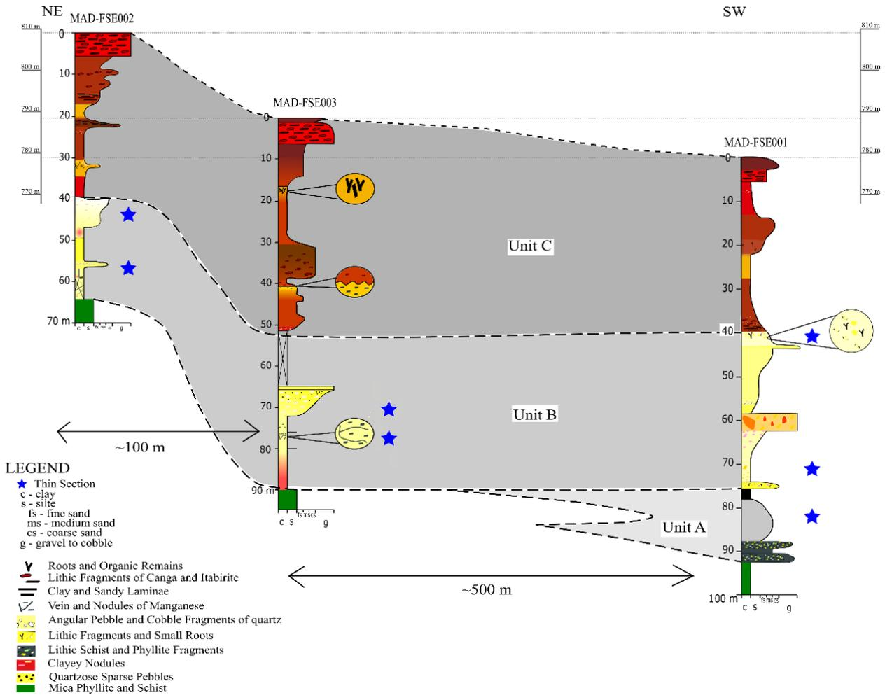
**Figure 8.** Drill hole profile description for MAD-FSE001, MAD-FSE002, and MAD-FSE003. Drill hole profiles are with individualized intervals, some remarkable features, and their correlations. The colors used are as similar as possible to the real core sample.
