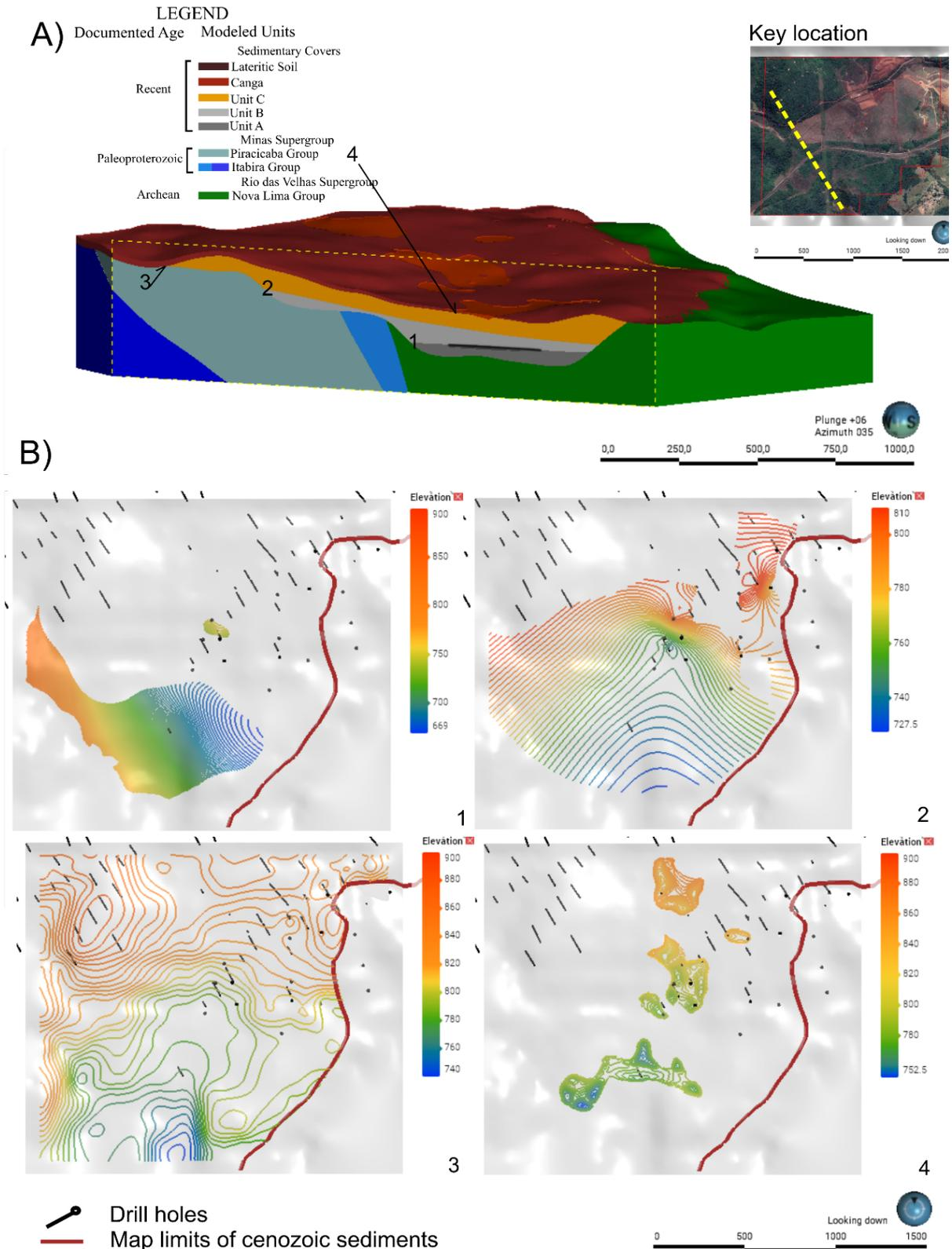
**Figure 11.** Modeled simulations of the Bandeira Basin. (A) Section of the geological model, considering the criteria and interpretation presented in this chapter; (B) contour map of the contact of the main sedimentary units identified in Bandeira Basin, presenting the contact between Units A and B in B1; contact between Units B and C in B2; contact of lateritic soil in B3 and contact of canga units in B4.
