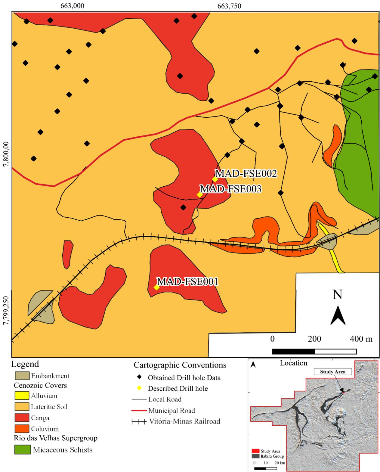
**Figure 2.** Simplified geological map of the Bandeira basin area highlighting the drill hole database.
