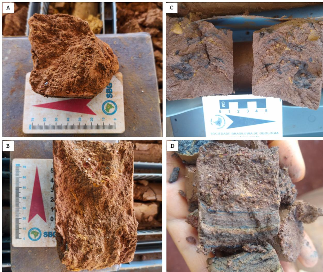
**Figure 5.** (A) Sand clayey matrix, with pebbles of canga and laterite; (B) CGSLith massive clayey matrix, with quartzose and lithic fragments; (C) CGSLim massive colluvium with clay to silty matrix, pebble-sized grain surrounded by goethite and some hematite silt widespread; (D) colluvium with planar bedding, with massive and laminated strata, rich in manganese, hematite, and quartz sand-sized grain and a few lithic fragments.
