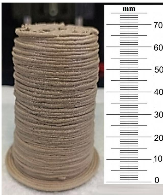
Figure 8: Image of cylindric geopolymer sample printed using metakaolin from batch 2, 0.05% of PP fibers, and 7.46 M alkaline solution.
