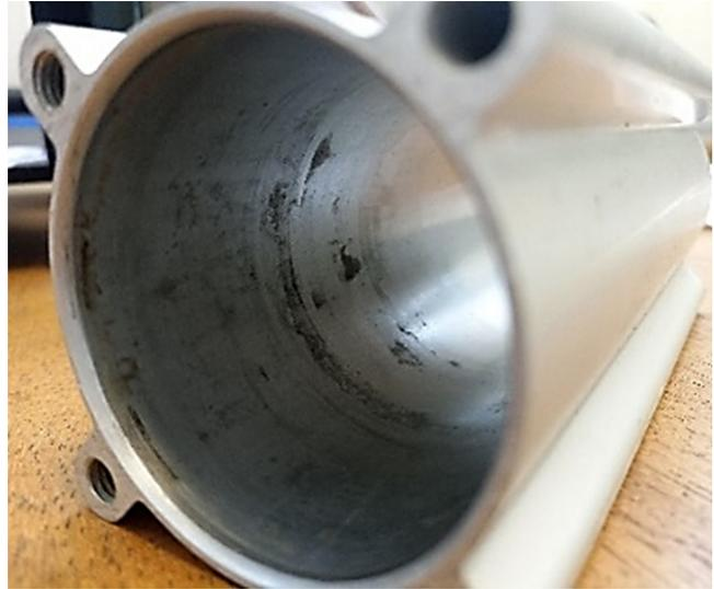
Figure 2: Image of aluminum pneumatic reservoir chemically affected by the geopolymer.
