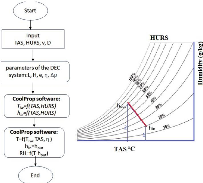
Figure 3 – Direct cooling pad in the psychrometric chart and flowchart of simulation parameters.
