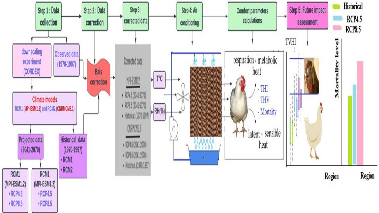
Figure 2 – Conceptual flowchart illustrating the methodology adopted for the evaluation of historical and future comfort conditions, as well mortality levels of broiler chickens when adopting a DCP system.
