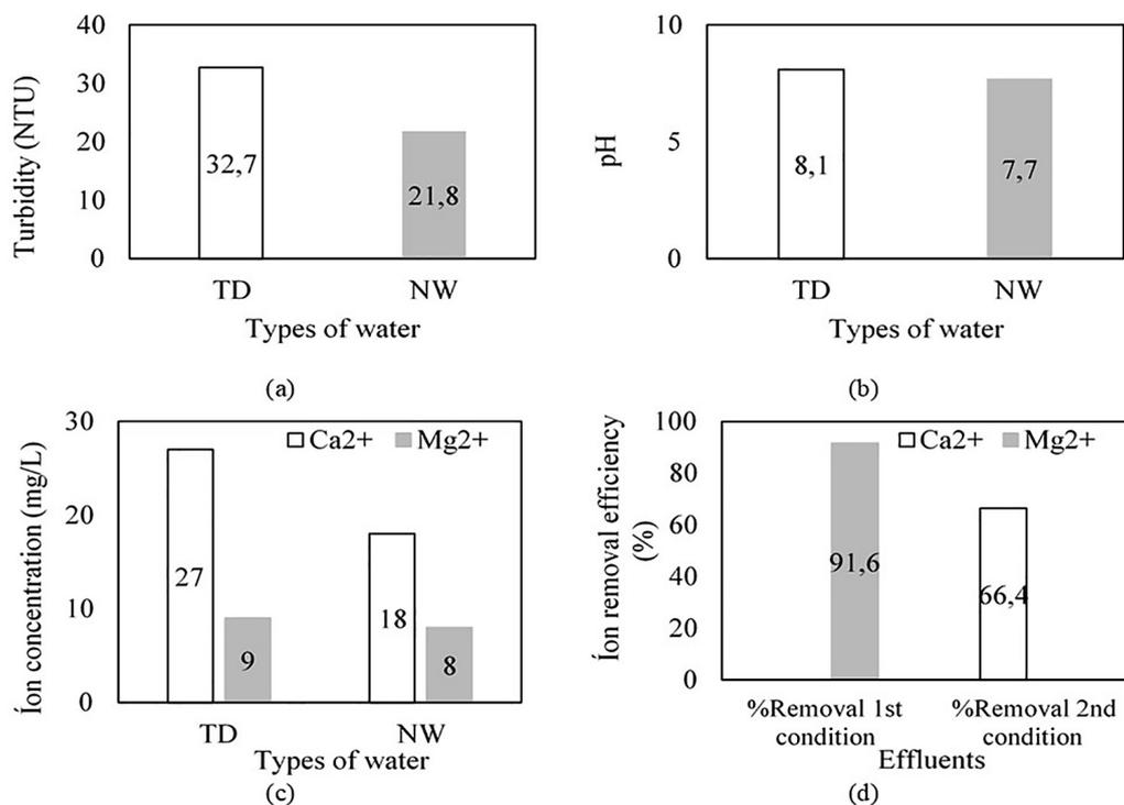
**Figure 1:** Characterization of TD effluent and NW by (a) turbidity (NTU), (b) pH, (c) ion concentration of  $\text{Ca}^{2+}$  and  $\text{Mg}^{2+}$  (mg/L), and (d) ion removal efficiency of  $\text{Ca}^{2+}$  and  $\text{Mg}^{2+}$  (%) from the SE effluent by DAF.
