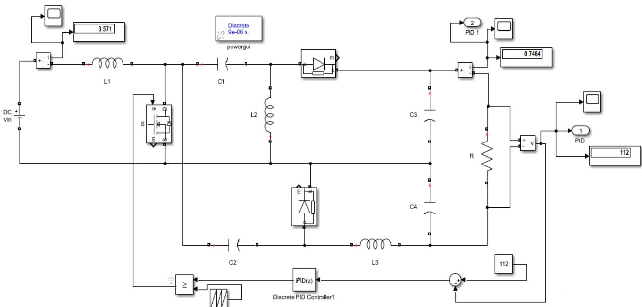
**Figure 3.** MATLAB / SIMULINK model of the proposed integrated DC-DC converter with PID controller
