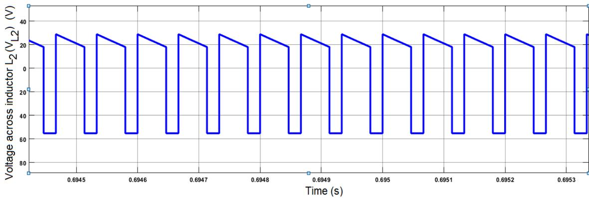
Figure 11. Voltage across inductor  $L_2$  ( $V_{L2}$ )
