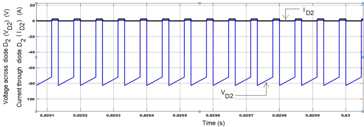
**Figure 18.** Voltage across diode D2 ( $V_{D2}$ ) and Current through diode D2 ( $I_{D2}$ )
