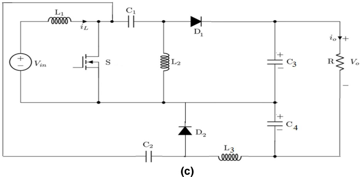
**Figure 1.** Topologies of DC-DC converter - **(a).** Conventional SEPIC converter, **(b).** CUK converter, **(c).** Proposed integrated converter.
