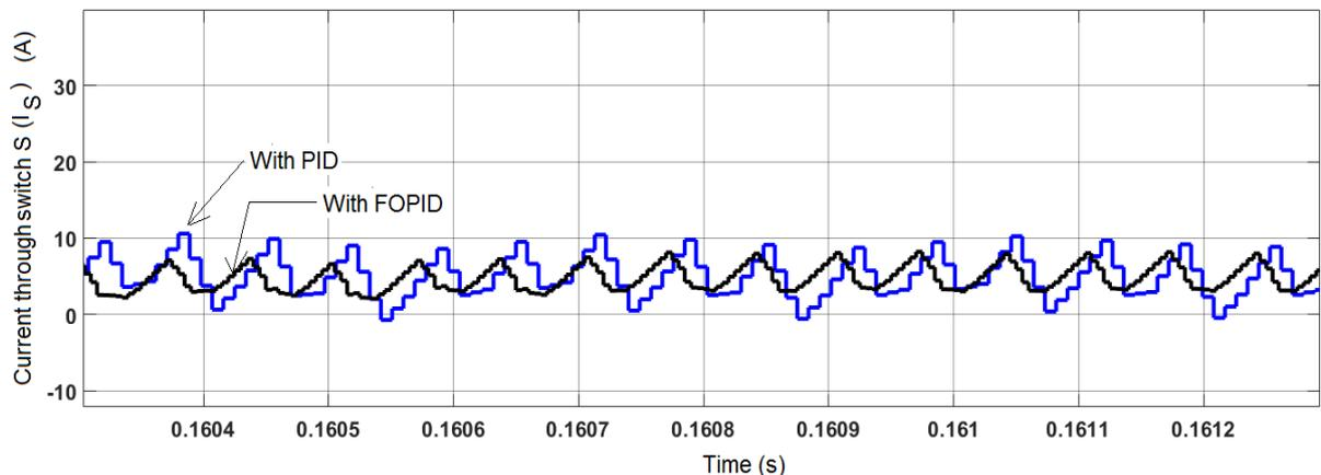
**Figure 20.** Current stress of switch S ( $I_s$ )
