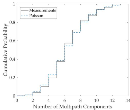
Fig. 12. Cumulative distribution function of the number of multipath.
