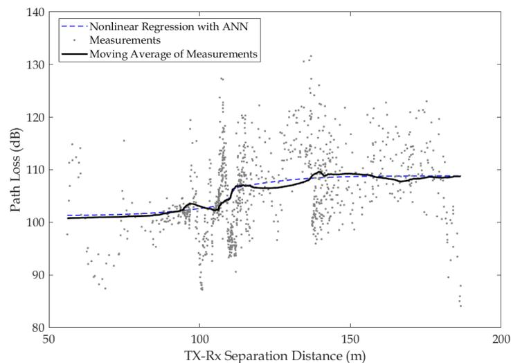
Fig. 9. Result of models fitted by ANN regression with two neurons in the hidden layer.
