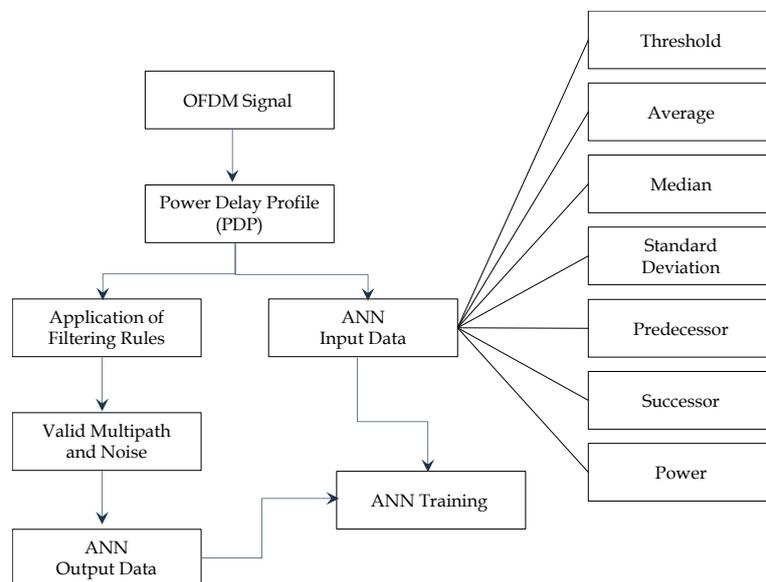
Fig. 3. Stages of ANN input and output preprocessing.
