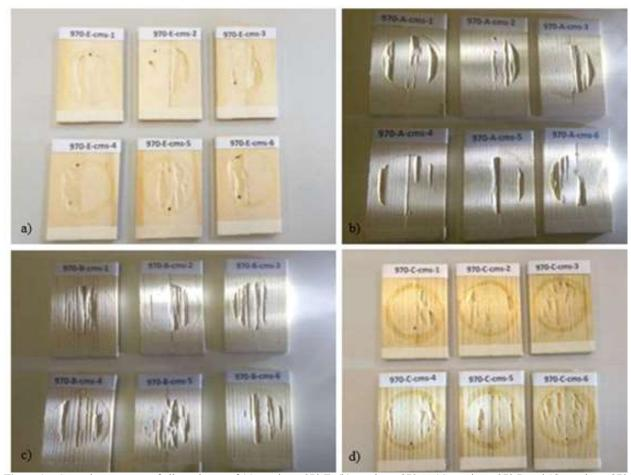
Figure 1 – General appearance of all specimens of (a) specimen 970 E; (b) specimen 970 A; (c) specimen 970 B and (d) specimen 970 C - after exposure to dry wood termite attack, for a period of 45 days: detail of wear caused by termites. Source: Technological Research Institute (IPT) test report N°. 1 136 740-203.
